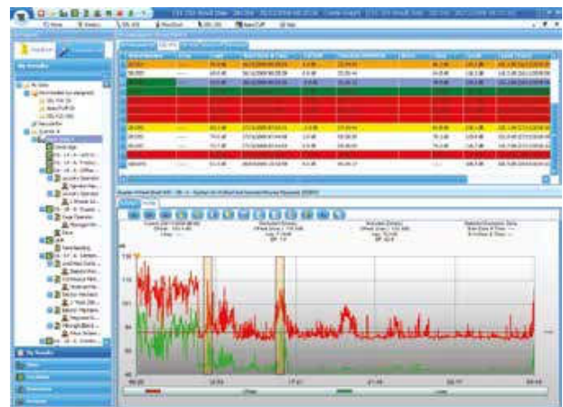
Tree style database of results with colour coding for exceeded noise action levels
